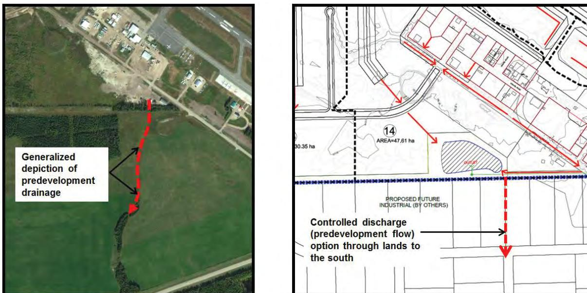
Figure ST-2: Controlled Discharge Option for Sub-catchment #14.
