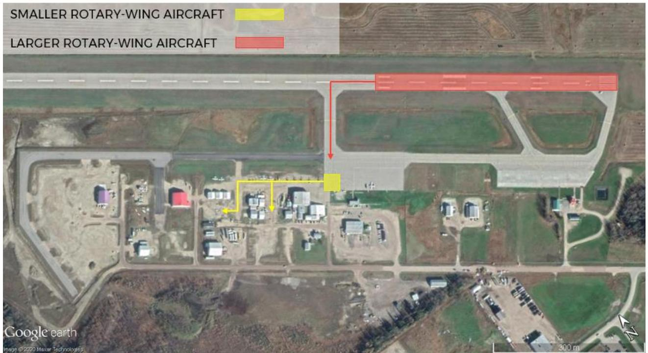
**Figure 6.4: Potential Traffic Paths for Smaller vs. Larger Rotary-Wing Aircraft**
